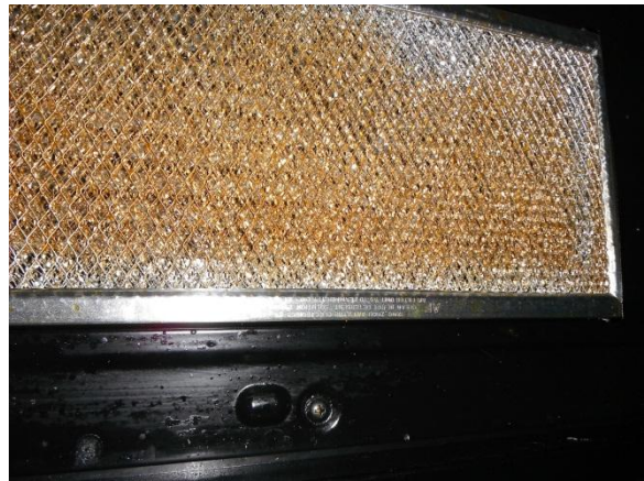
Microwave Filter is Dirty
